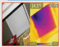
Our Infrared Camera allows us to see things that cannot be seen with the naked eye such as areas of energy loss, moisture in
