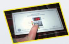
We offer electronic radon testing utilizing a Sun Nuclear 1027 Professional Monitor. Additional charges apply.
