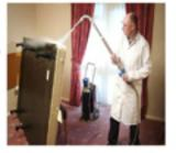
The Cryonite System releases CO2 as "snow" which, when applied to the infested sites, rapidly kills bed bugs, cockroaches and flour beetles on contact.
